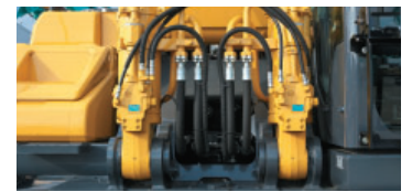
Boom, arm and jib holding valves Standard - to prevent boom or arm from falling if hose is damaged.
