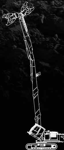
Ultra long attachment specification [11'6" (3.5m) boom insert]
