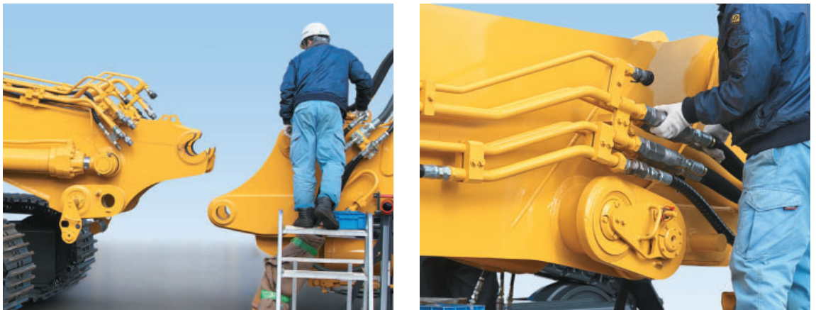
Piping connection: Hydraulic quick coupler system on the side of the boom.
