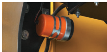
Travel alarm The alarm cautions workers in the area that the machine is traveling.
